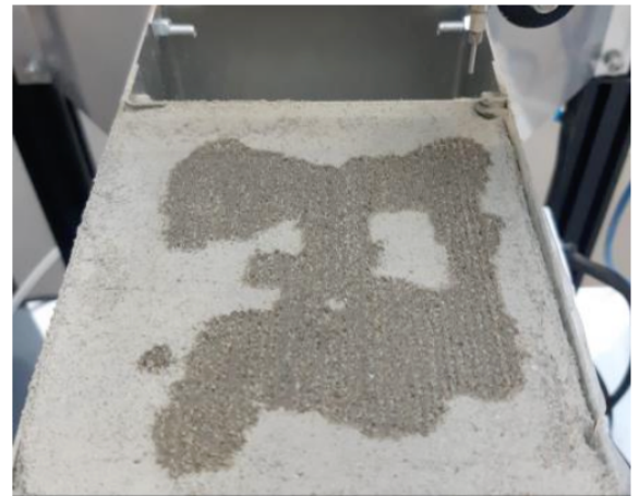
Image 23: Layer with added binder (source: Coastruction)
