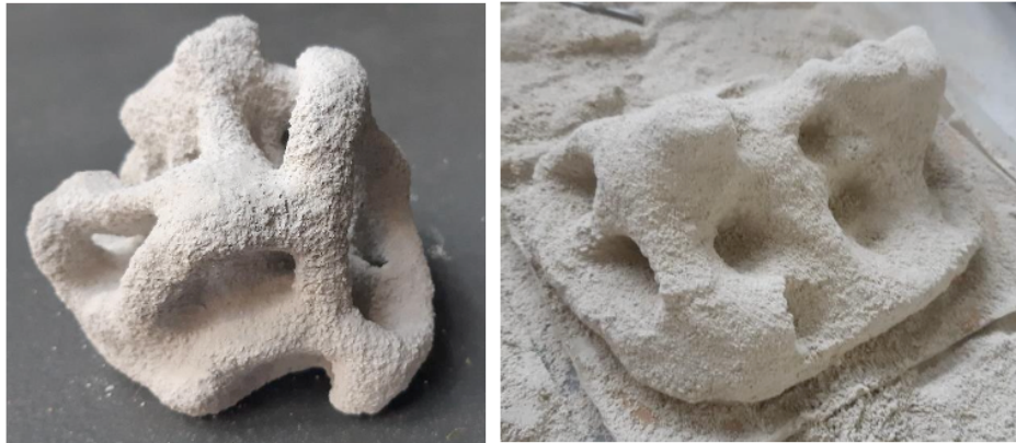
Image 27: Aragonite sand as aggregate (source: Coastruction)
