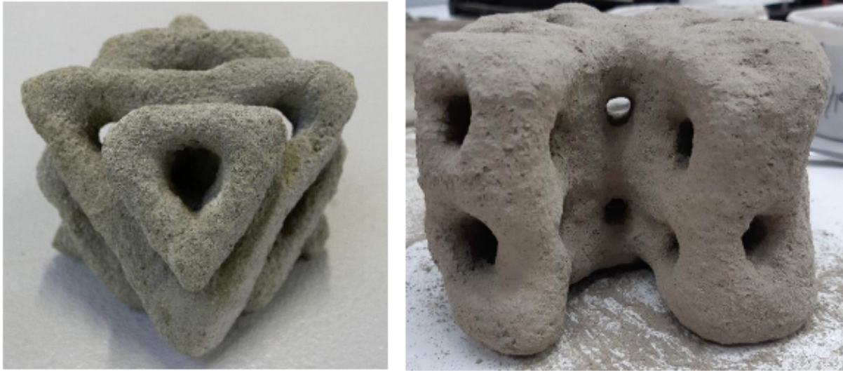
Image 30: Recycled concrete as aggregate (source: Coastruction)
