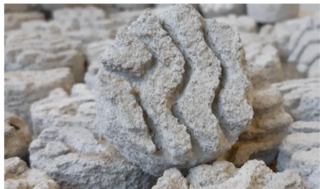
Image 26: Dolomite sand as aggregate (source: Coastruction)
