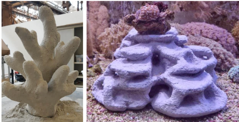
Image 28: Quartz sand as aggregate (source: Coastruction)
