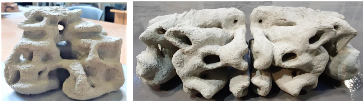
Image 29: Beach sand as aggregate (source: Coastruction)
