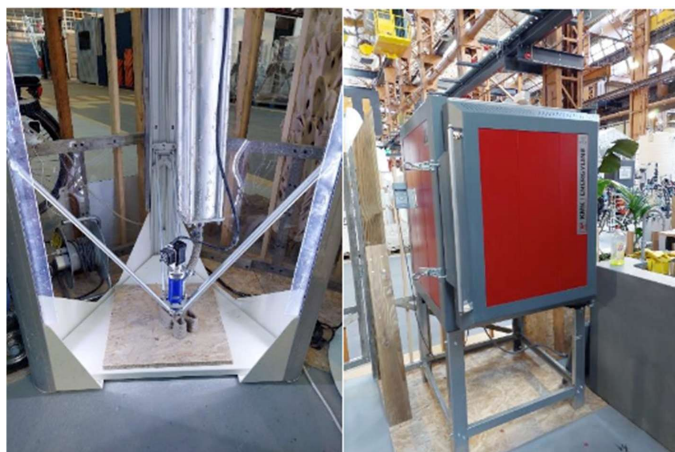
Image 37: Printing (left) and firing (right) (source: Matser, 2023)
