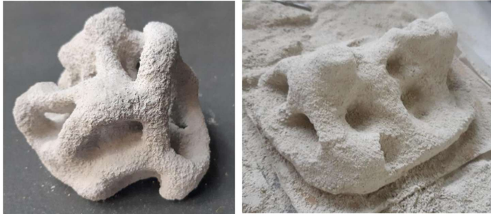
Image 27: Aragonite sand as aggregate (source: Coastruction)
