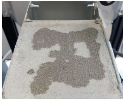
Image 23: Layer with added binder (source: Coastruction)
