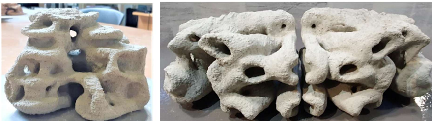
Image 29: Beach sand as aggregate (source: Coastruction)
