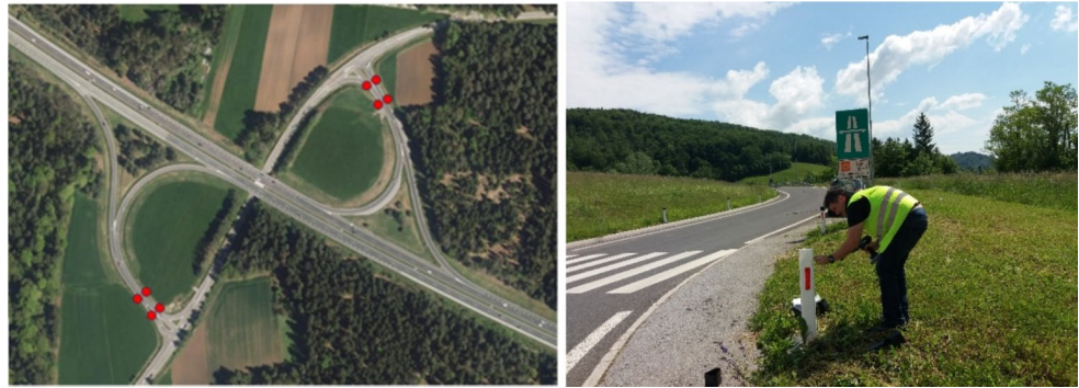
Fig. 1 One of the highway interchanges, showing general principle of installation of acoustic deterrents (red dots)
