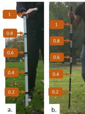
Fig. 1. (annex 3) Two examples of calibration poles. The top of each group of bands is at a known height above ground at 20 cm intervals. Heights above ground are indicated in metres, with the number of bands in each group indicating the height increment.
