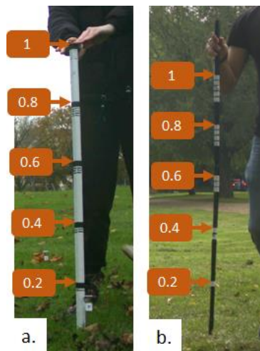
Figure 5. Two examples of calibration poles. The top of each group of bands is at a known height above ground at 20 cm intervals. Heights above ground are indicated in meters, with the number of bands in each group indicating the height increment.
