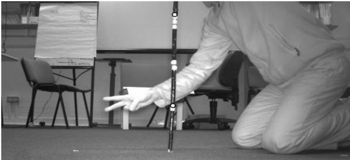
Fig. 5. (annex 3). A camera calibration image with pole in position 2 m from the camera.
