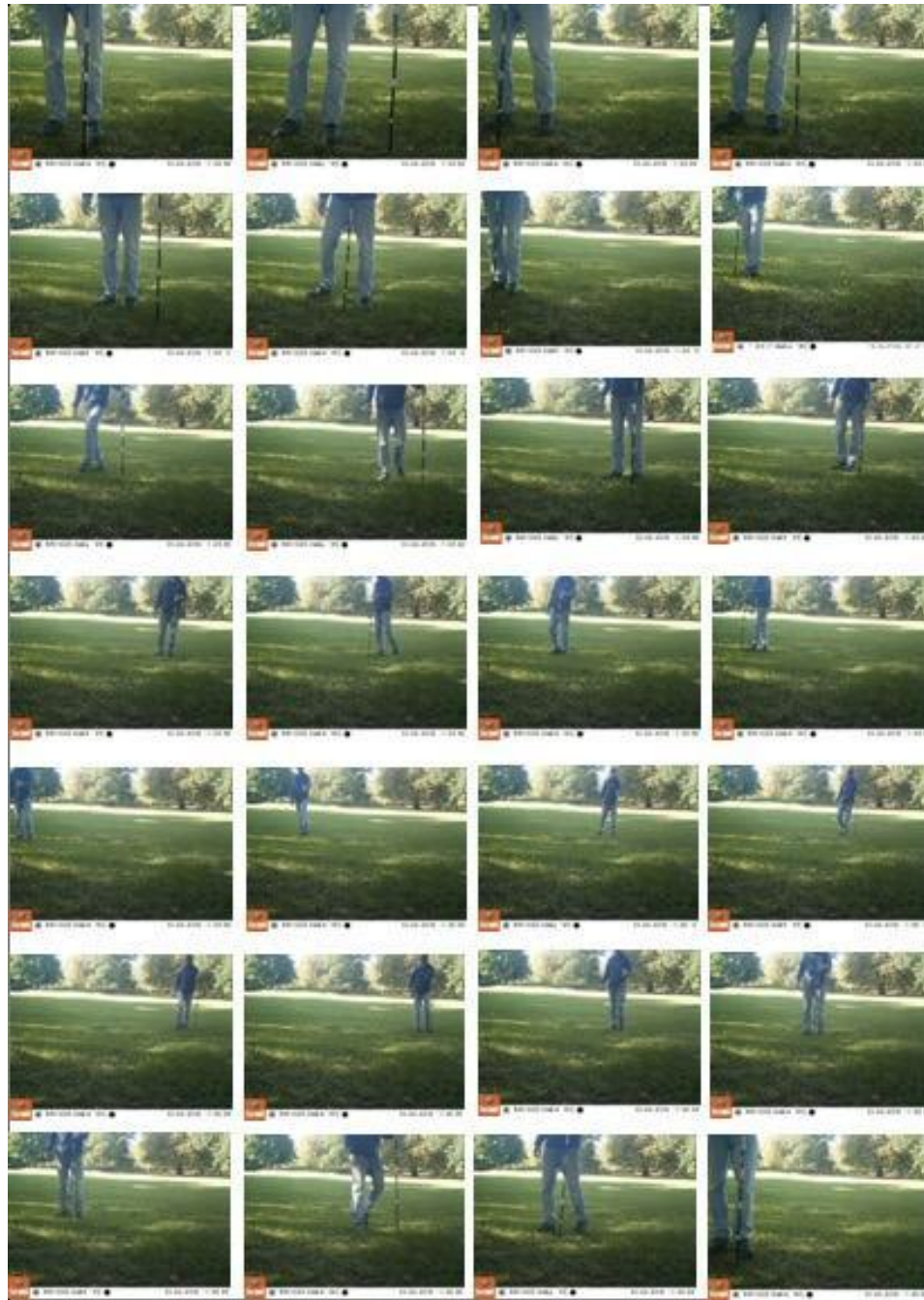
Fig. 3. (annex 3). A set of deployment calibration images showing 28 pole positions with good coverage of the detection zone.
